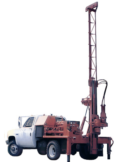
Typical truck-mounted drill
