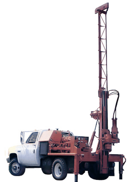
Typical truck-mounted drill
